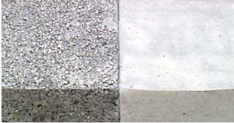
Figure 1.1: SRI of similar mixes of traditional concrete and pervious concrete (Haselbach et al. 2011)
