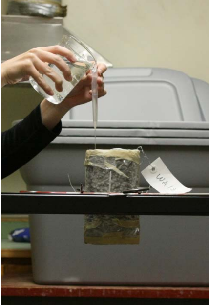
Figure 3.1: Rain water retention test
