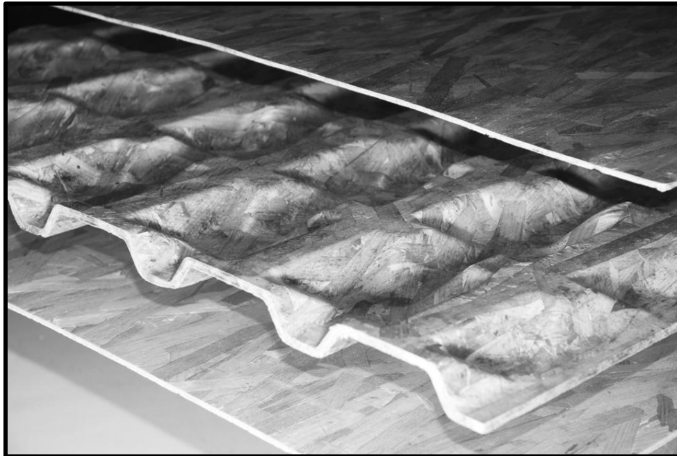
Figure 3.1. Exploded view of the hollow core panel. The three-dimensional hollow-core wood-strand composite sandwich panel was used as structural skins for this study. This sandwich panel took the place of the oriented strand board structurally skins typical used for structural insulated panels. Photo courtesy of the Composite Materials and Engineering Center – Washington State University.
