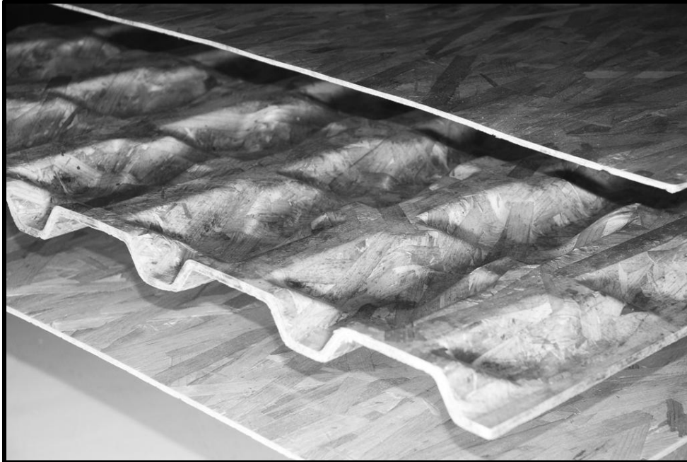
Figure 2.1. Exploded view of the hollow core panel. This photo depicts an exploded view of the HCP used as structural skins for the proposed wall assembly. The panel consists of a three-dimensional corrugated like hollow-core adhered to thin OSB skins. The continuous longitudinal ribbing shown can provide housing for utilities, insulation, or ventilation. Photo courtesy of the Composite Material and Engineering Center at Washington State University.
