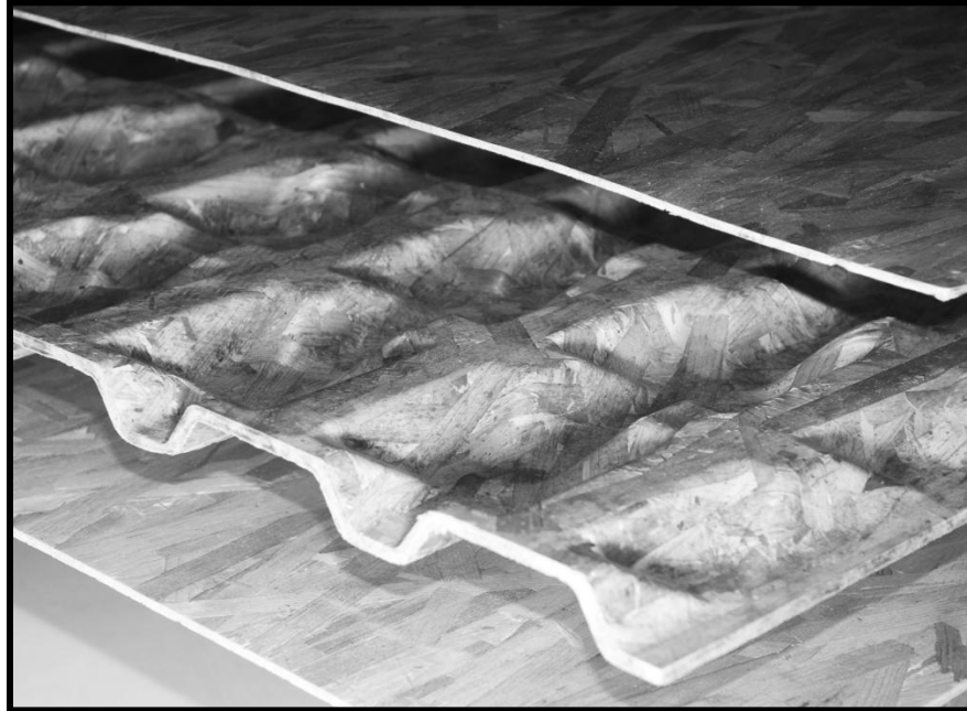
Figure1.1. Exploded view of the hollow core panel. The three-dimensional hollow- core wood- strand composite sandwich panel was used as structural skins for this study. This sandwich panel took the place of the oriented strand board structurally skins typical used for SIPs. Photo courtesy of the Composite Materials and Engineering Center – Washington State University.
