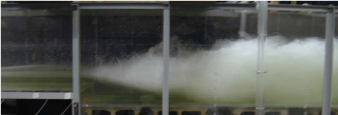
Weir Located 7 ft downstream from drop. Run # 87 Q = 7.2 cfs
