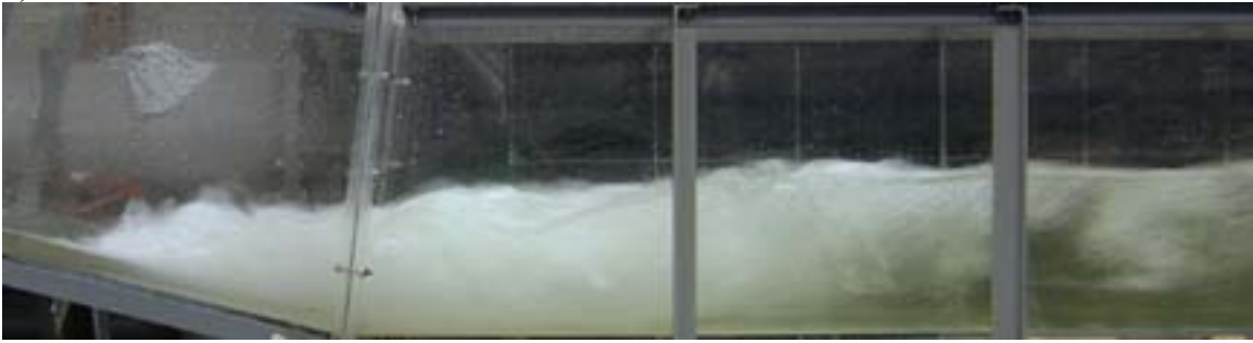
Figure 5. Design I Observed Jumps: a) Standing Wave L_w/y_2 = 0.9 b) Complete Jump L_w/y_2 = 5 , and c) Submerged Jump L_w/y_2 = 9 .
