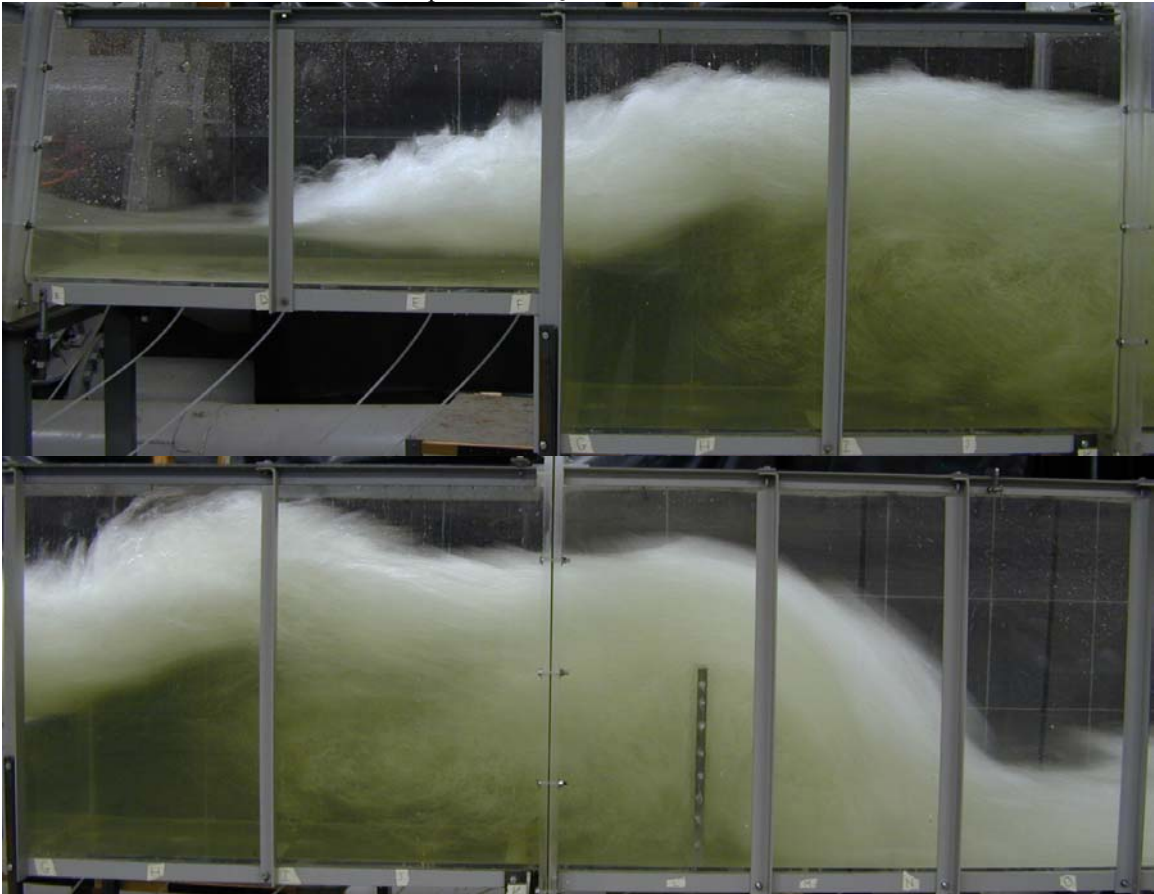
Weir Located 5 ft downstream from drop. Run # 25 Q = 8.1 cfs
