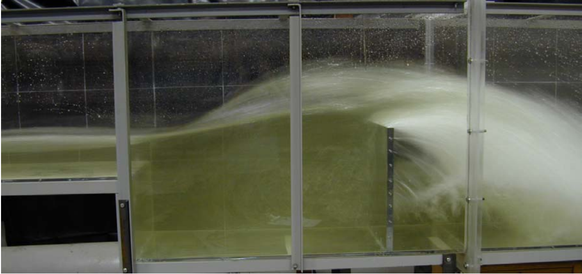
Weir Located 3 ft downstream from drop. Run # 9 Q = 8.2 cfs
