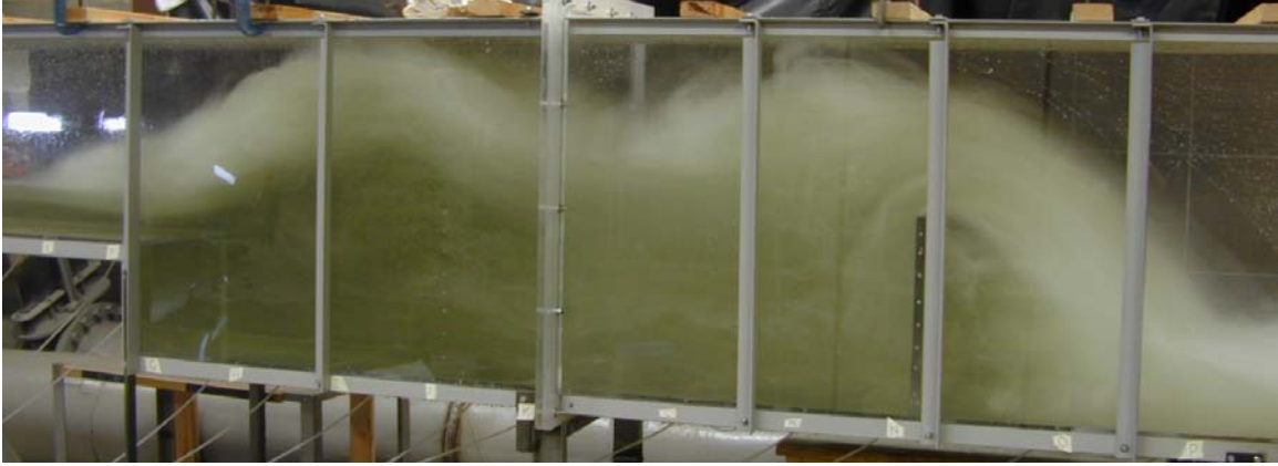
Weir Located 7 ft downstream from drop. Run # 16 Q = 8.3 cfs
