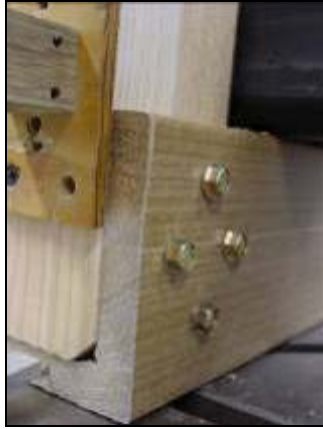
Figure 2.9 Typical connection test geometry
