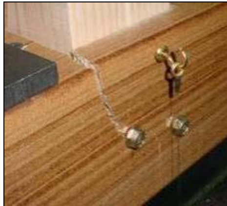
Figure 3.9 Typical component test flexural failure at end stud slot
