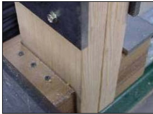
Figure 3.6 Perpendicular-to-extrusion screw reinforcement between flange and webs
