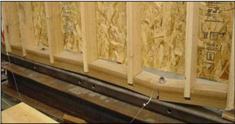
Figure 4.14 Overall PP10 hollow sill plate behavior (load being applied from right side)
