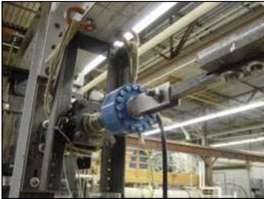
Actuator connection to top load beam
