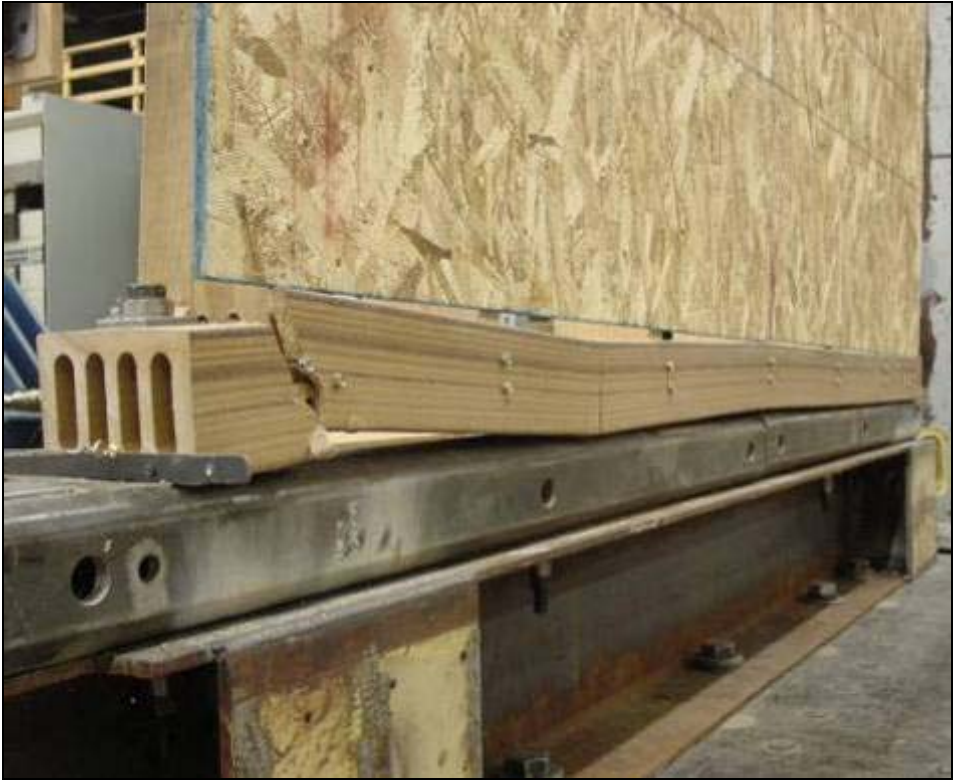
Figure B.2 Test PP10-M sill failure and overall behavior
