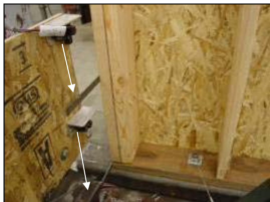
Stud and Sill Displacement Measures—North End
