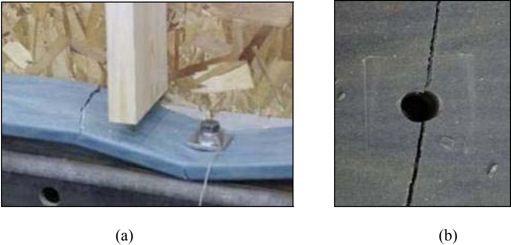
Figure 4.6 Sill failures: (a) Sill bending and flexural cracking at anchor bolt nearest loaded end stud, and (b) Plate washer indentation and anchor bolt hole size increase from bearing
