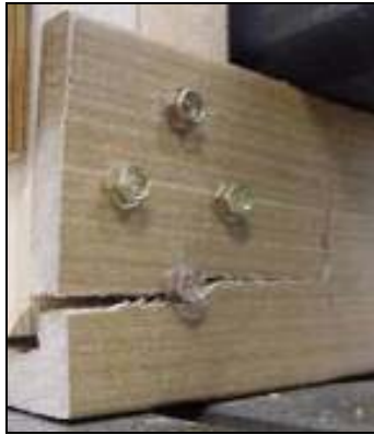
Figure 3.1 Typical failure path in connection tests (Specimen 4 shown)
