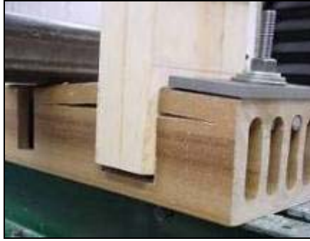
Figure 3.2 Failure perpendicular-to-extrusion between flange and webs from uplift force transferred to dowels
