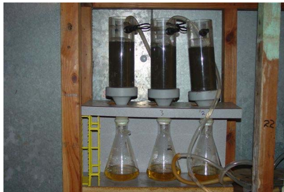
Figure 12A. Laboratory Soil Column Setup
