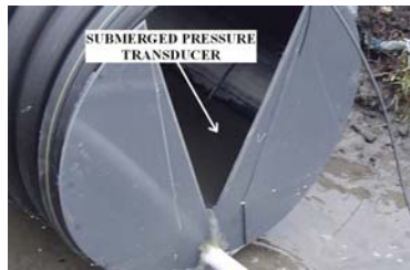
Figure2. Spokane Culvert Pressure Transducer Field Setup.
