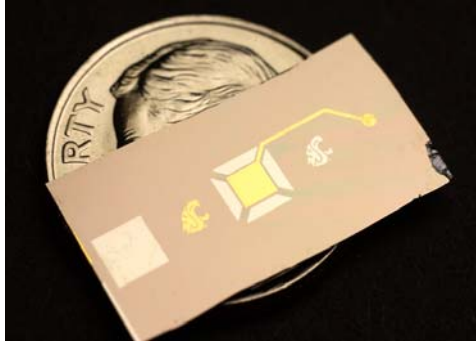
Figure 4.2.1 5x5mm thin film PZT sample
