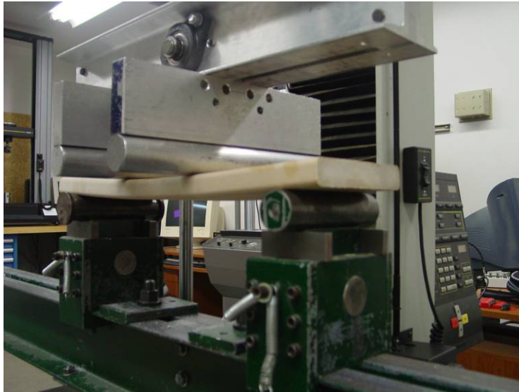
Figure 3.1. Typical flexure test setup for WPC deck boards.
