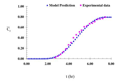
Fig. 6: Model predictions versus experimental results for DBT obtained from Worch (2004).
