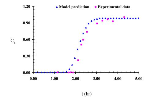
Fig. 5: Model predictions versus experimental results for 2,4,6-TCP obtained from Rahman et al. (2003).
