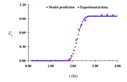
Fig. 4: Model predictions versus experimental results for 2-M-4,6-DNP obtained from Rahman et al. (2003).
