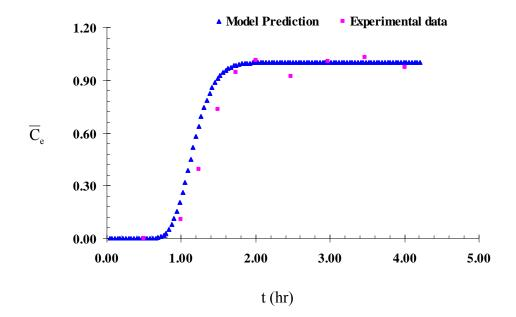
Fig. 7: Model predictions versus experimental results for PCP obtained from Worch (2004).
