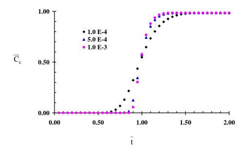
Fig. 2: Effect of varying film transfer coefficients, in cm  $s^{-1}$ , on model prediction.
