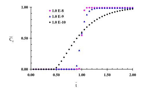
Fig. 3: Effect of varying diffusion coefficients, in  $cm^2 s^{-1}$ , on model prediction.
