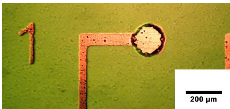
Figure 3.5 A corner of the electrode array, covered with SU-8 except directly over the pad
