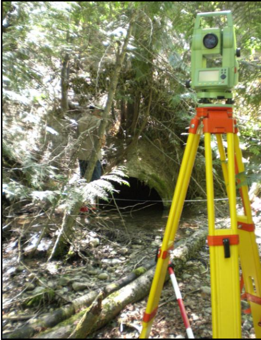
Figure C6.1: Downstream end of the Matsen Creek culvert including the Total Station utilized during survey work
