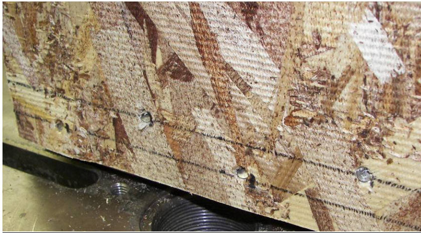
Figure 3-8 , Sheathing nails pulling through OSB
