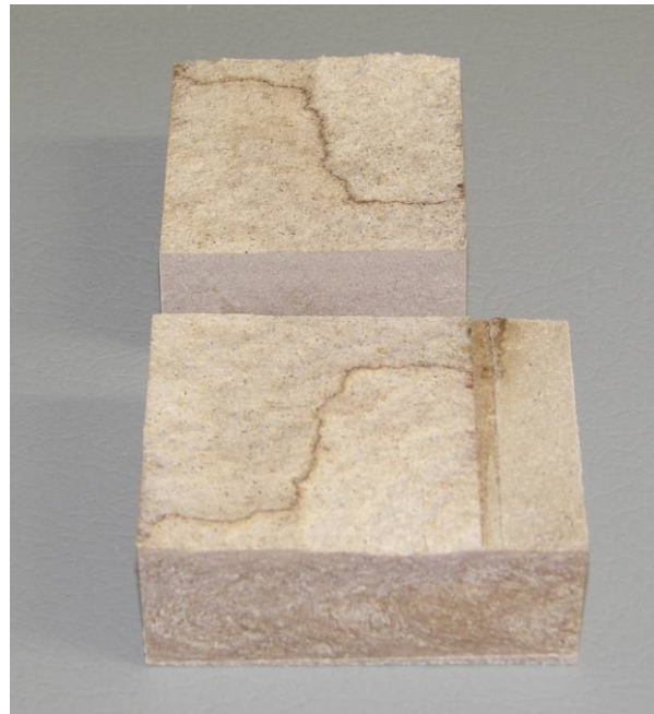
Figure 1-6 Glue-line shear block failure
