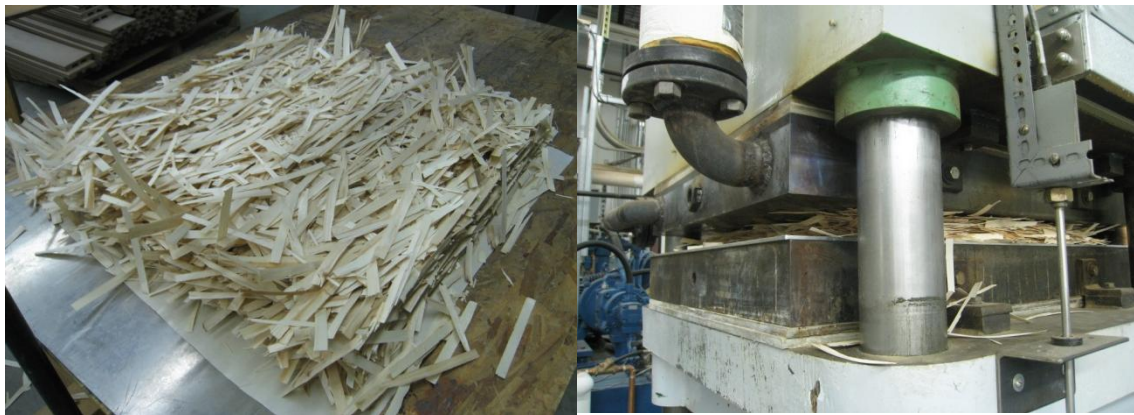
Figure 3-3 Loose mat and hot pressing
