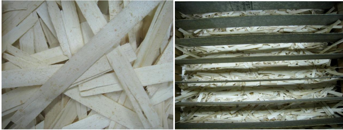
Figure 3-2 Resinated strands distributed through forming box
