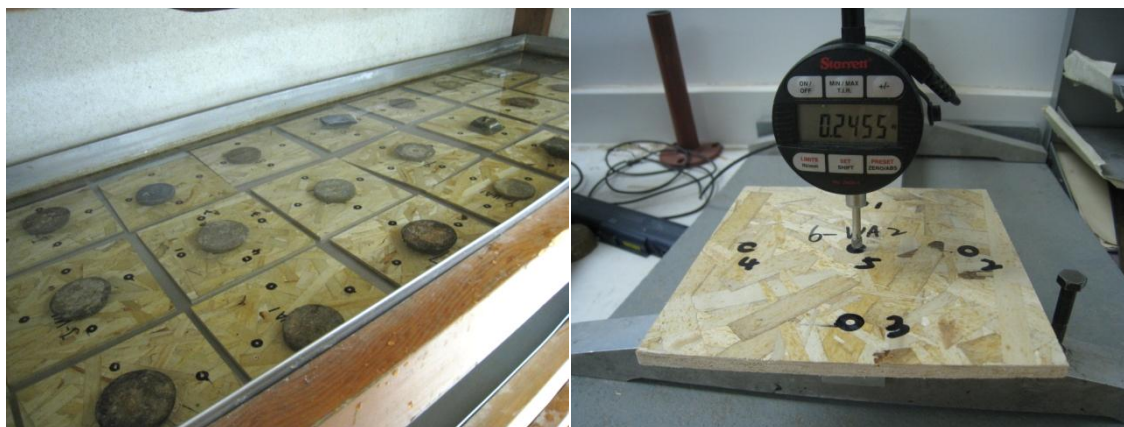
Figure 3-7 Water submersion (Left) and five-spots thickness measurement (Right)
