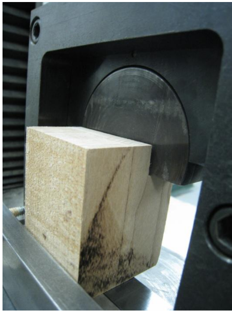
Figure 2-9 Glued wood specimen for neat wood shear block test
