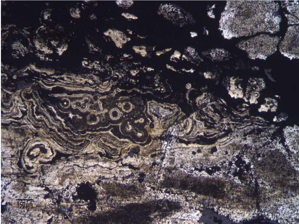
YS-08-JM152: Fractured, botryoidal, colloform marcasite (copper-colored) healed by brecciated pyrite.
