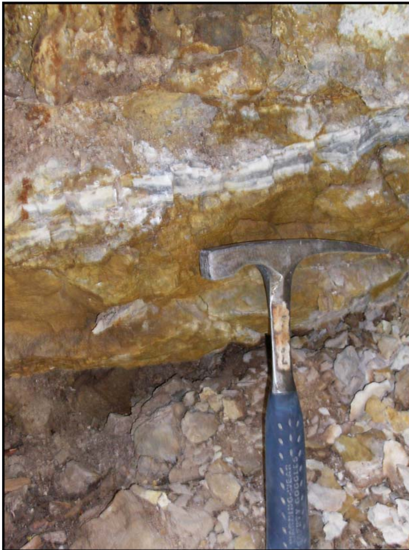
Figure 18: Colloform silica vein. Saunders (1990) noted in the Sleeper deposit Au is often associated with the lighter bands, while the darker bands are barren.
