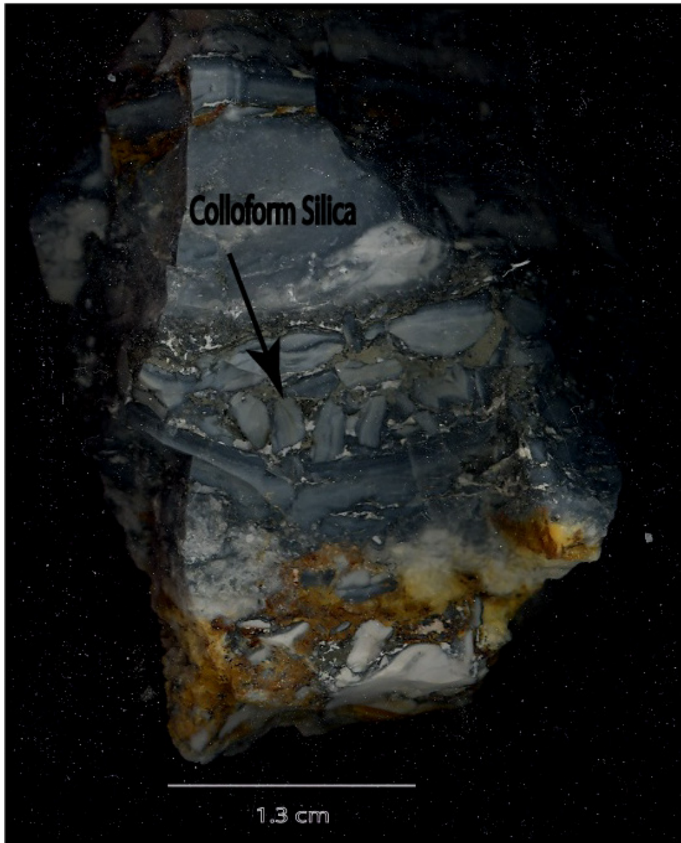
Figure 32: Brecciated hand sample YS-08-JM20. Breccia include milled fragments of colloform silica.
