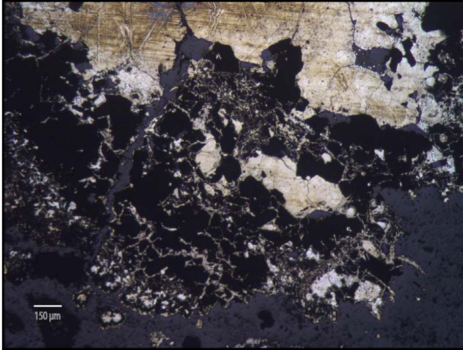
Figure 30: Micrograph of crackle breccia in sample YS-08-JM155 #2. Sample contains angular, clast-supported fragments (dark) healed by sulfides. Reflected; cross-polarized light.
