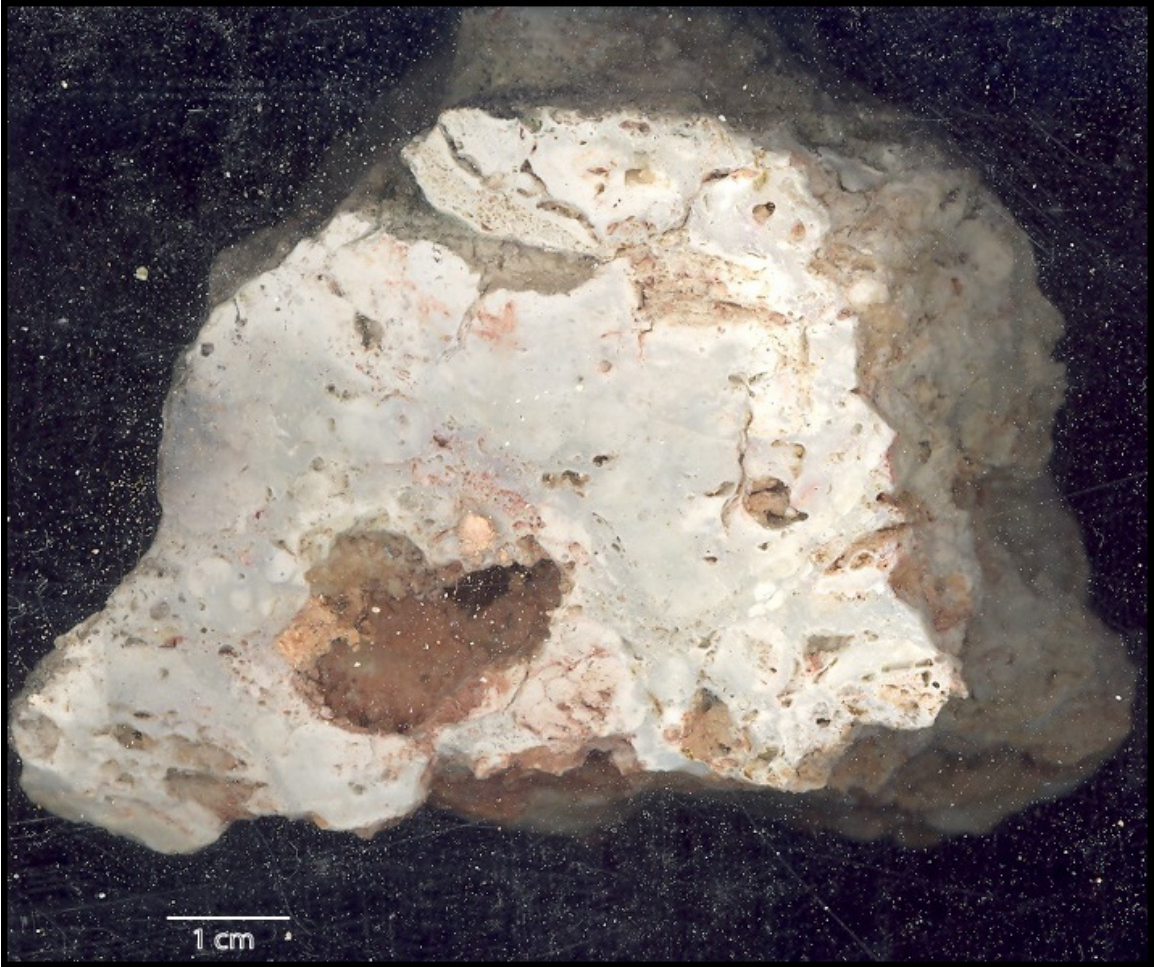
Figure 14: Silicified hand sample YS-08-JM125. Sample contains vuggy silica and the large vug contains drusy quartz.
