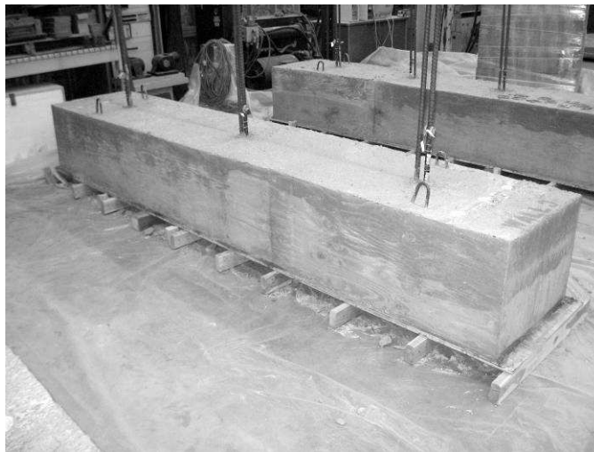
Figure A-4: Foundation with flexural reinforcement at 48 in. (1219 mm).
