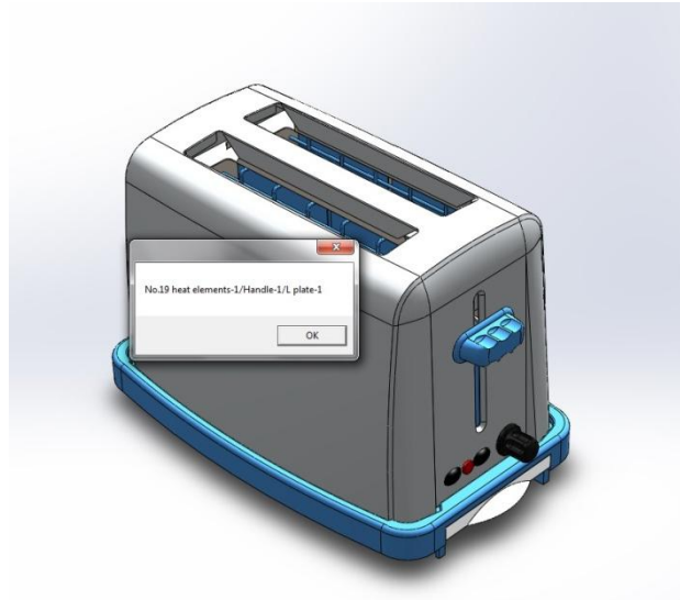
Figure 5.3 Highlighted part and notification dialog box for the standard toaster CAD assembly model.
