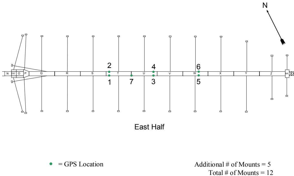
Figure 2.11 - Locations of GPS Receivers on EPFB, Configuration 2
