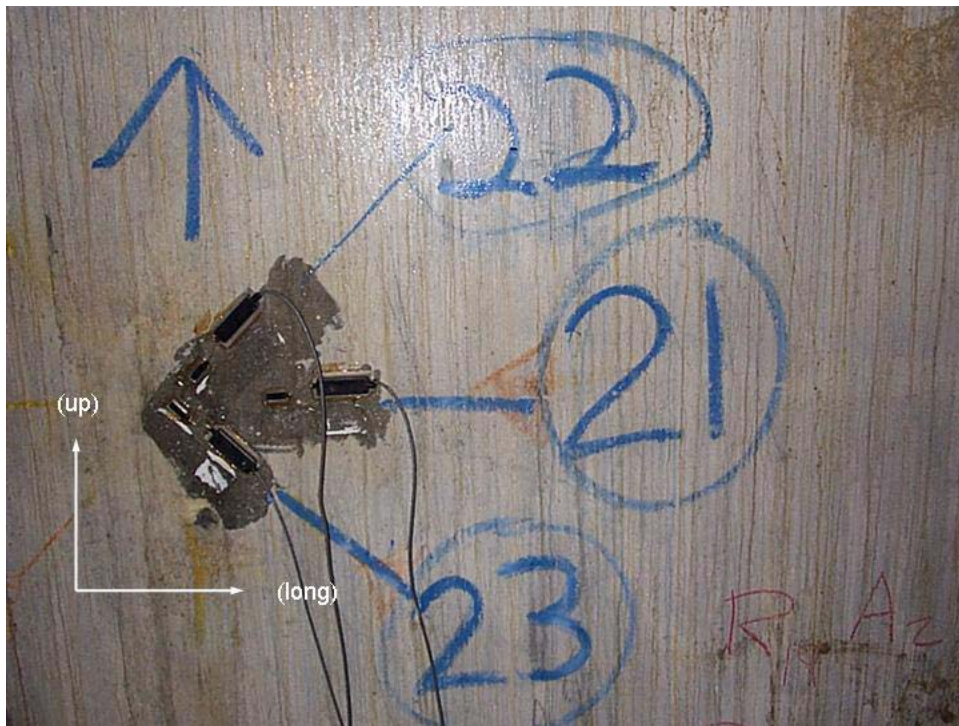
Figure A.13 – Strain Gages # 13 (flexure), #22 & #23 (shear)
