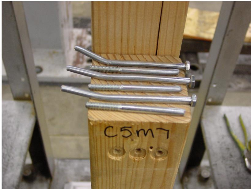
Figure 4.15: Photograph of bolt failure. Mode IV yield; three rows of one bolt.
