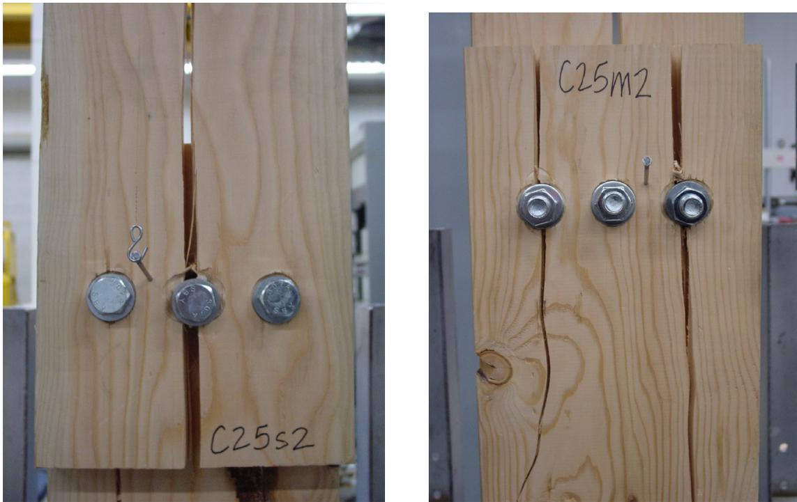
Figure 4.3: Photograph of different types of row splitting for a single specimen. Mode II yield; three rows of one bolt.
