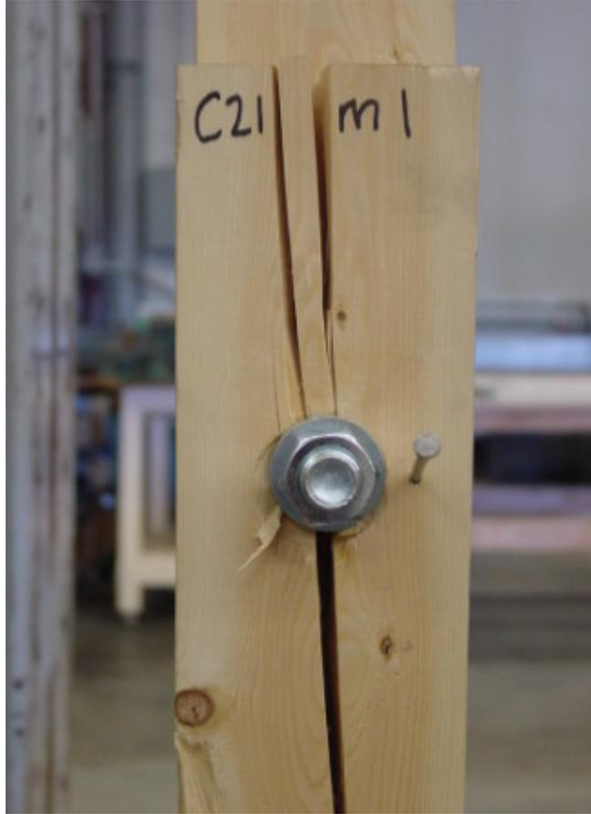
Figure 4.1: Photograph of Mode II splitting/plug shear failure.
