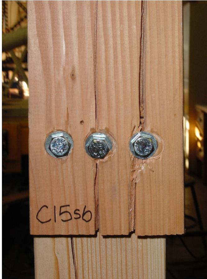
Figure 4.9: Photograph of typical splitting. Mode III<sub>s</sub> yield; three rows of one bolt.
