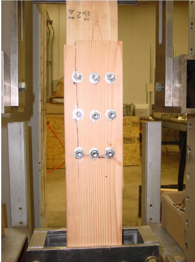
Figure 4.5: Photograph of group tear-out. Mode II yield; three rows of three bolts.
