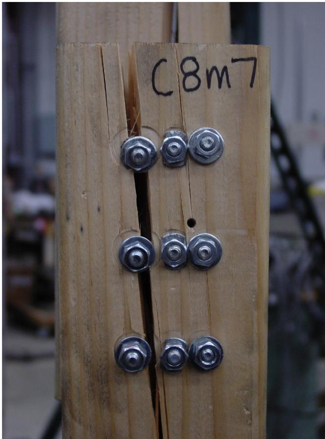
Figure 4.17: Photograph of spitting. Mode IV yield; three rows of three bolts.
