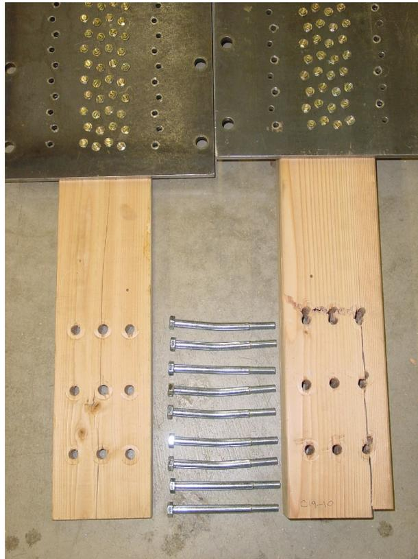
Figure 4.11: Photograph of group tear-out. Mode III<sub>s</sub> yield, three rows of three bolts.
