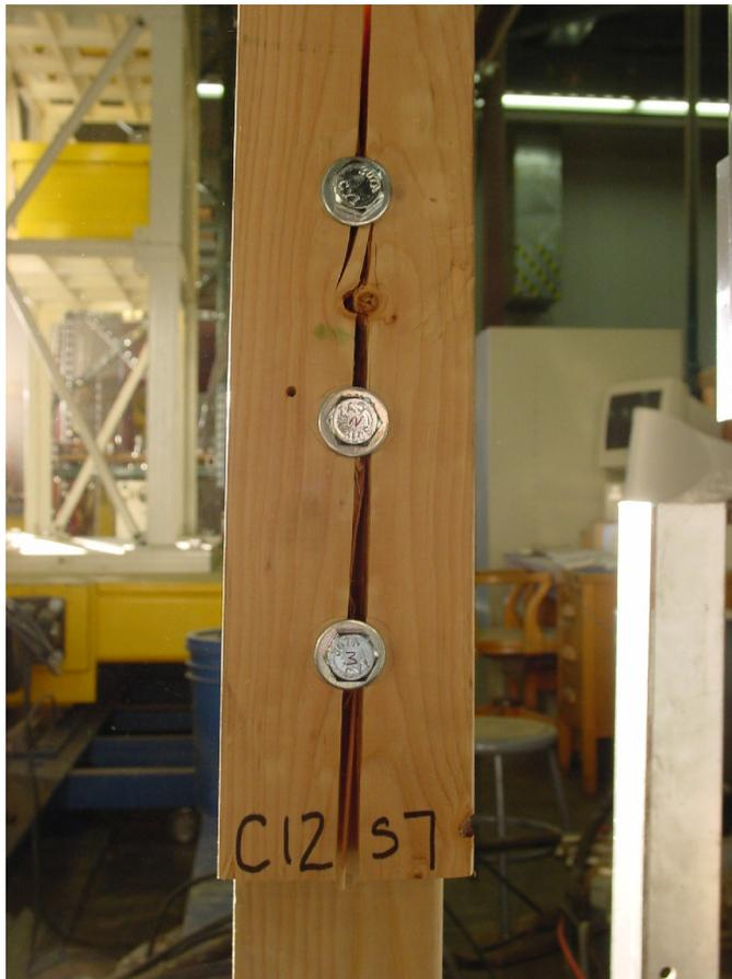
Figure 4.7: Photograph of typical splitting failure. Mode III<sub>s</sub> yield; one row of three bolts.
