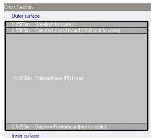
Figure III.5.1.3.1 - DesignBuilder cross section of SH roof.
